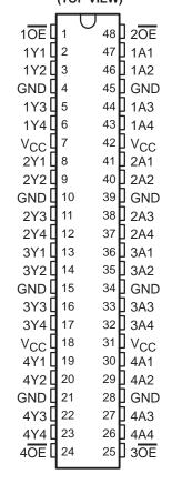
These devices can be used as four 4-bit buffers, two 8-bit buffers, or one 16-bit buffer. They provide true outputs and symmetrical active-low output-enable  $(\overline{OE})$  inputs.
